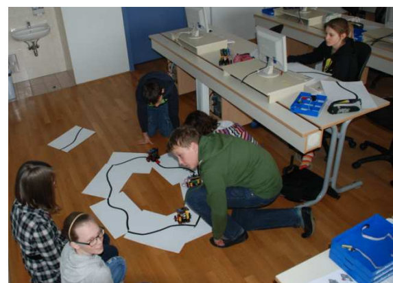
Fig 4: Testing and developing the program for line follower robot.
